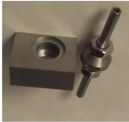
Figure 2. Photographs of cathode and anode of magnetron for SPS with active cooling.
