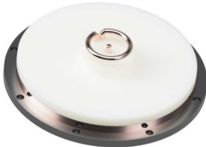
Figure 9: Rendering of a cell module concept with the coil implanted in the cathode and the modified design incorporated into a cell stack. Colours do not indicate materials.
