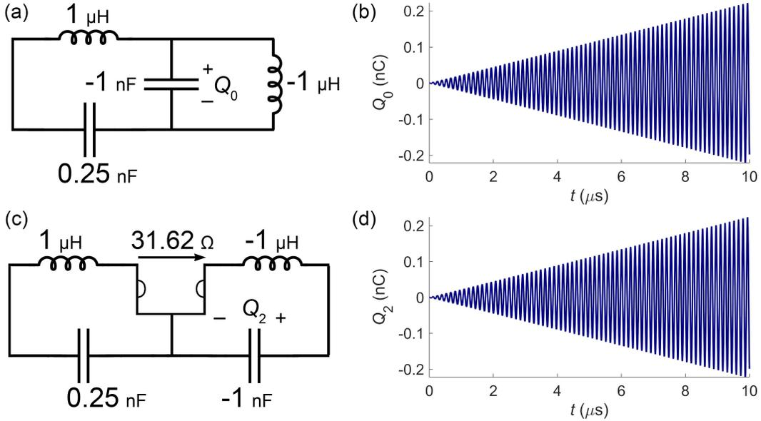
FIGURE 7. Comparison between the time-domain simulation results of (a) the PRC and (c) the GNC with the proposed equivalent element values. The stored charges in the capacitor with the negative capacitance in (b) the PRC  $Q_0(t)$  and (d) the GNC  $Q_2(t)$  under the EPD condition and by applying the equivalency conditions.
