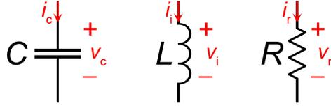
FIGURE 8. Capacitance, inductance and resistance symbols and the relevant parameters in the electric circuits.
