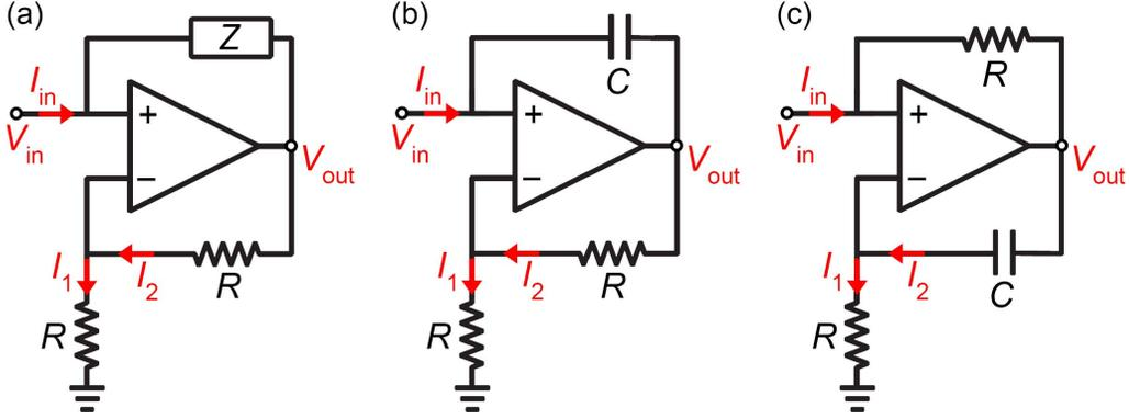
FIGURE 9. Opamp-based negative (a) impedance converter, (b) capacitance converter, (c) inductance converter.
