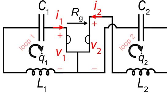
FIGURE 4. The two-loop nonreciprocal circuit coupled by an ideal gyrator. For specific combinations of values  $L_1$ ,  $C_1$ ,  $L_2$ , and  $C_2$ , the evolution matrix of the nonreciprocal circuit develops a degeneracy, and its nontrivial Jordan canonical form consists of exactly two Jordan blocks of size 2. A change in the sign of  $R_g$  is equivalent to reversing the gyration resistance direction (indicated by the arrow below  $R_g$ ) in this circuit.
