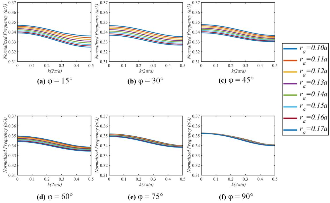
**Fig. 3:** The variation of normalized frequency of the 3<sup>rd</sup> band with the radius of auxiliary rod ranging between  $r_a = 0.10a - 0.17a$  for the auxiliary rod angles of (a)  $\varphi = 15^\circ$ , (b)  $\varphi = 30^\circ$ , (c)  $\varphi = 45^\circ$ , (d)  $\varphi = 60^\circ$ , (e)  $\varphi = 75^\circ$  and (f)  $\varphi = 90^\circ$ . The radius of cavity and the distance between cavity and auxiliary rod are taken as  $r_c = 0.35a$  and  $\Delta = 0.10a$ , respectively.
