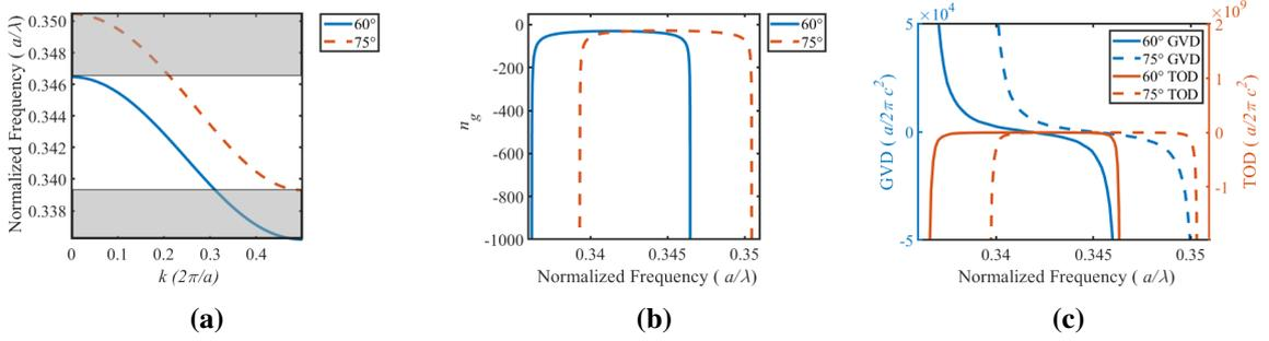
**Fig. 4:** (a) Band structure and (b)  $n_g$ , (c) GVD and TOD values of  $3^{rd}$  band for auxillary rod angles  $\varphi$  of  $60^\circ$  and  $75^\circ$  structures showing mini-band gap.
