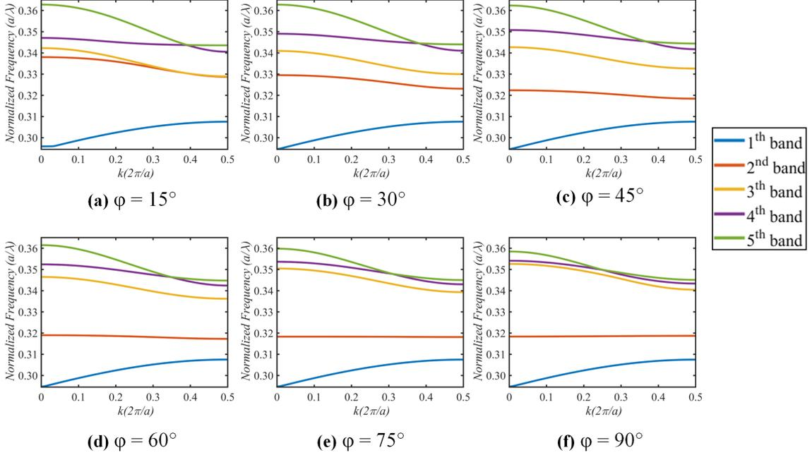
**Fig. 2:** The band structure of low-symmetry cavity structure with the auxiliary rods of radius  $r_a = 0.14a$  at the angles of (a)  $\varphi = 15^\circ$ , (b)  $\varphi = 30^\circ$ , (c)  $\varphi = 45^\circ$ , (d)  $\varphi = 60^\circ$ , (e)  $\varphi = 75^\circ$  and (f)  $\varphi = 90^\circ$ . The radius of cavity and the distance between the cavity and the auxiliary rod are taken as  $r_c = 0.35a$  and  $\Delta = 0.10a$ , respectively.
