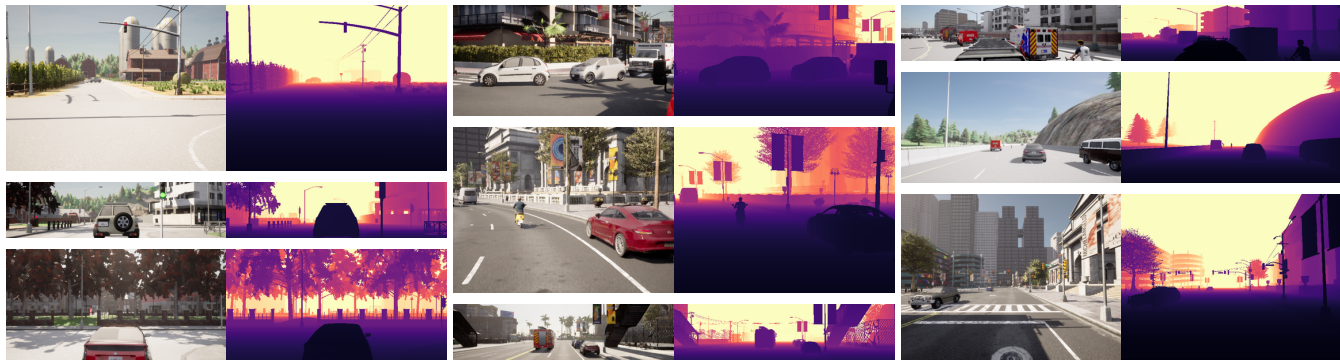
Fig. 9: Images and corresponding ground-truth depth maps from our publicly available dataset created in the CARLA simulator. Samples are acquired with a diverse set of vehicle-camera systems in urban, rural and highway environments.
