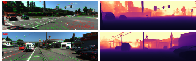
Fig. 17: MOFT [19] feature matches and corresponding depths on the KITTI-360 sequences. GenDepth depth estimation enhances feature tracking and enables robust matching with a high percentage of inliers (green matches) after RANSAC optimization.
