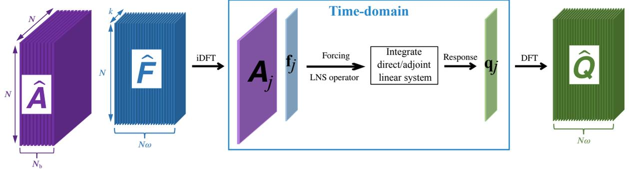
Figure 2: Schematic of the action of  $\mathbf{H}$  with streaming DFT/iDFT to transform between the Fourier and time domains.
