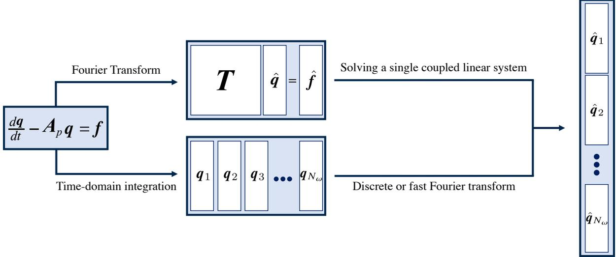
Figure 1: Flowchart depicting the action of  $\mathbf{H}$  on a forcing comprised of  $N_\omega$  frequencies within the RSVD-LU (top route) and the RSVD- $\Delta t$  (bottom route) algorithms. Both routes produce the same result, but the bottom route is computationally advantageous for large systems.
