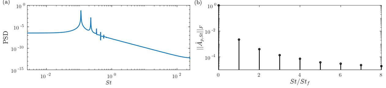
Figure 8: Airfoil test case: (a) the PSD spectrum based on transverse velocity at  $(x/L_c, y/L_c) = (3.0, -0.43)$ . (b) The normalized Frobenius norm of  $\hat{\mathbf{A}}_{p,St}$  up to the eighth harmonic.
