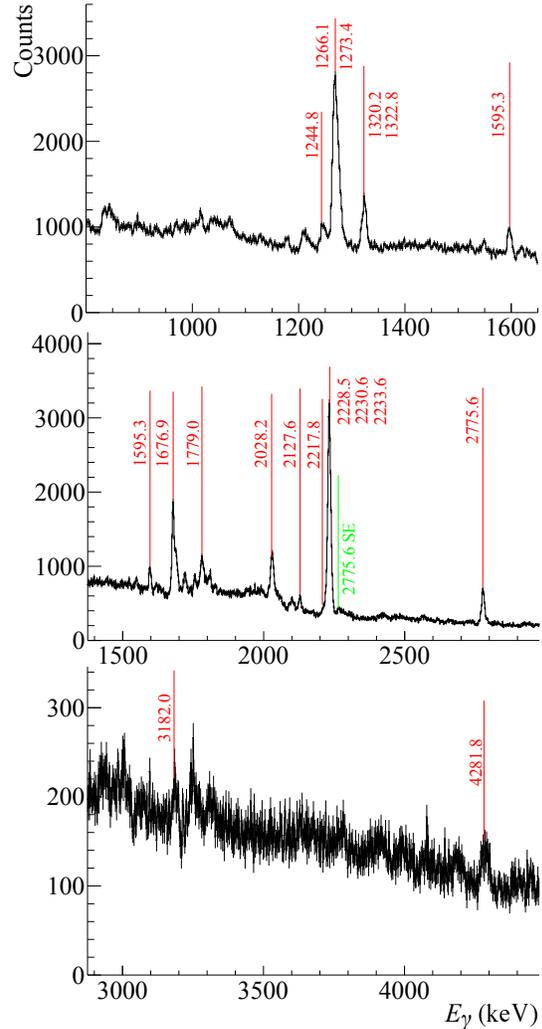
Fig. 10. Energy spectrum of  $\gamma$ -quanta in the range 800–4500 keV, measured with the HPGe detector during the irradiation of a sulfur sample. Green line – single escape peak. Identification of the  $\gamma$ -peaks was performed via TalysLib, see details in text.
