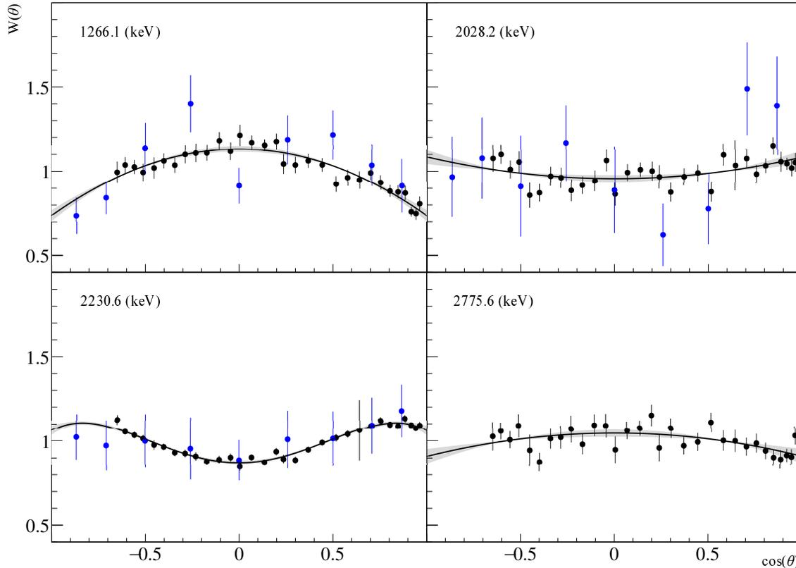
Fig. 11. Angular distributions of  $\gamma$ -quanta from radiative transitions in sulfur. The energies correspond to the strongest transition in the unresolved peaks. Black dots show the data of this work, blue – data from [30]. The black solid line is the polynomial approximation of our data by the Legendre polynomials according to
