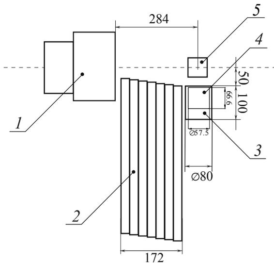
Fig. 1. Scheme of the TANGRA setup with the HPGe detector in the reaction plane: 1 – neutron generator ING-27, 2 – lead shielding, 3 – housing of the HPGe detector, 4 – HPGe crystal, 5 – sample. The axis of the experimental setup is indicated by a horizontal dashed line. The tritium-enriched target is marked with an asterisk. All dimensions are given in mm.
