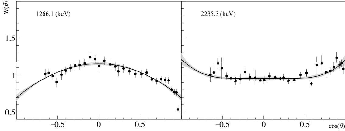
Fig. 9. Angular distributions of  $\gamma$ -quanta from radiative transitions in phosphorus. The energies correspond to the strongest transition in the unresolved peaks. Black dots show the data of this work. The black solid line is the approximation of these data by the Legendre polynomials according to formula (5). The grey areas show the 95% confidence interval of the approximation made, taking into account the statistical and systematic errors of the angular anisotropy parameters.
