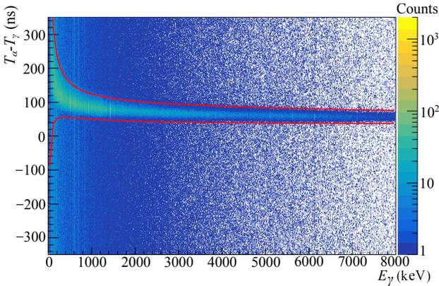
Fig. 5. Full TOF-Energy spectrum from measurement with HPGe detector. Color represents the number of counts. Coincidence window is marked by solid lines.
