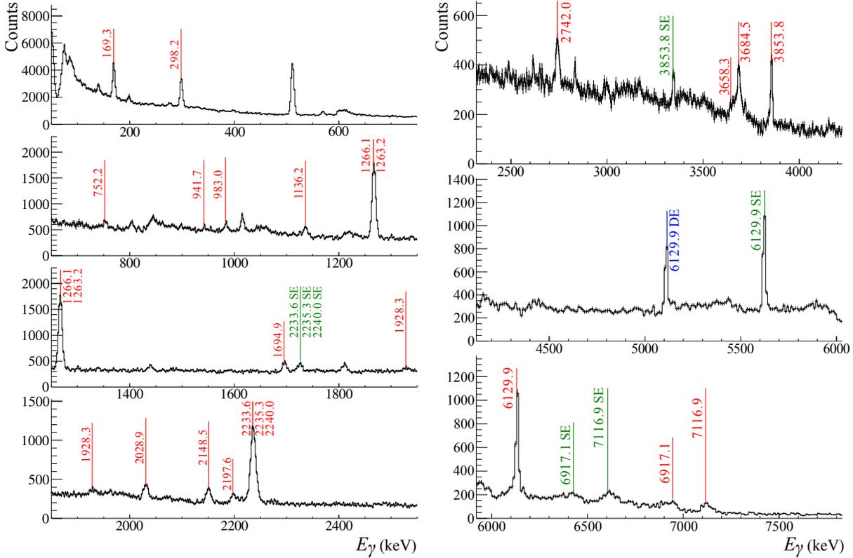
Fig. 7. Energy spectrum of  $\gamma$ -quanta from the  $P_2O_5$  sample in the range 50–7600 keV, measured by the HPGe detector. Position of  $\gamma$ -peaks identified by TalysLib and attributed to reactions with oxygen or phosphorus are marked by red lines. Single escape (SE) and double escape (DE) peaks of strong  $\gamma$ -transitions are marked by green and blue lines, respectively. The peak at 511 keV corresponds to electron-positron annihilation processes.
