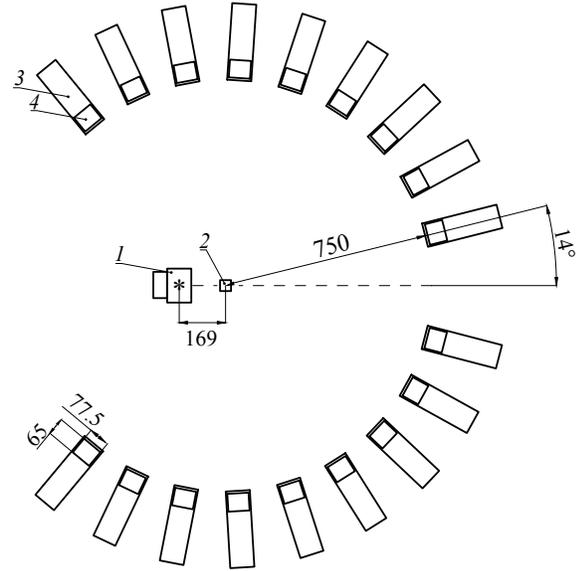
Fig. 2. Scheme of the TANGRA setup with BGO detectors in the reaction plane: 1 – portable neutron generator ING-27, 2 – sample in the center of Romasha  $\gamma$ -ray registration system, 3 – BGO detector housing, 4 – BGO crystal. The symmetry axis of the experimental setup is indicated by a horizontal dashed line. The tritium-enriched target is marked with an asterisk. All dimensions are given in mm.
