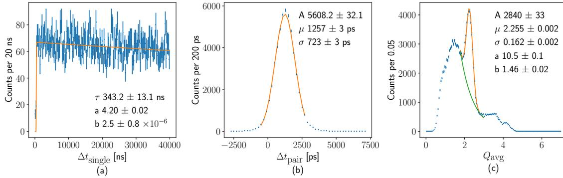
**Figure 3.** Determination of various performance metrics shown on the example of the TOFPET2c system data. (a) Time interval between subsequent events in a channel. The average time interval is 419  $\mu$ s. (b) Arrival time difference between two channels on opposite ends of a fiber. (c)  $^{22}\text{Na}$  spectrum from a single LYSO:Ce,Ca fiber, constructed as a geometric mean of the signals registered on its two ends.
