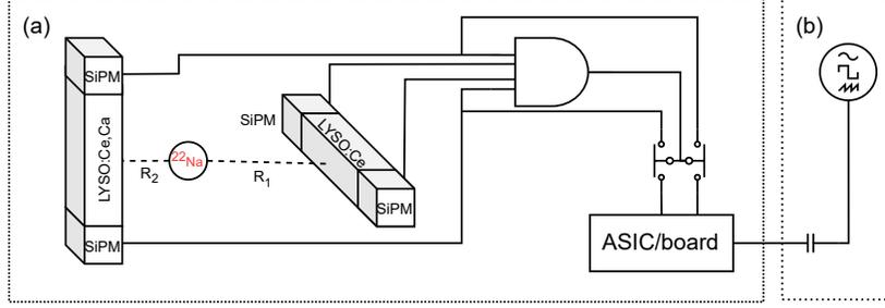
**Figure 2.** Detection test setups used in the study. The details vary slightly between different readout systems.  $R_1 \approx 61.4$  mm is the distance from the source to the reference detector and  $R_2 \approx 30.5$  mm is the distance from the source to the middle of the LYSO:Ce,Ca fiber. Setup (a) is used for dead time, coincidence time and energy resolution measurements, and setup (b) for efficiency and dynamic range studies.
