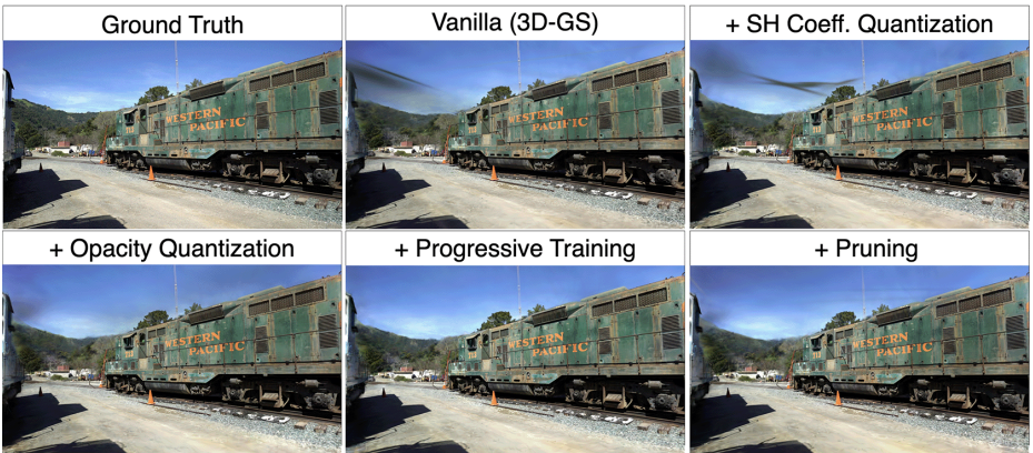
Fig. 7: Opacity quantization and progressive retraining removes floaters. Adding the pruning stage does not significantly affect quality while improving efficiency.
