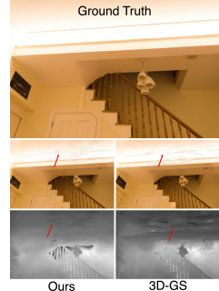
Fig. 5: 3D-GS produces artifacts (right) at various scene locations (arrow) while our rendering produces more scene consistent depth (left).
