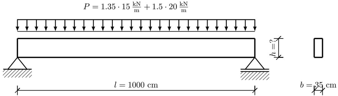
**Fig. 1** Geometry of the design problem of a bending beam with a constant distributed load (dead load and live load with safety factors of 1.35 and 1.5) and a rectangular cross section. The design variable, beam height is denoted by  $h$
