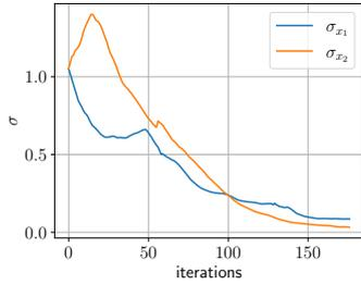
**Fig. 18** Evolution of the standard deviations  $\sigma$  of the design variables to highlight convergence of the optimization process. We note that the design variables are transformed and scaled in the optimization procedure
