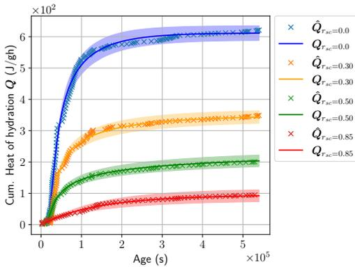
**Fig. 16** Predictive performance of the learned model corresponding to the hydration process. The solid line is the predictive mean and the shaded area is  $\pm 2 \times$  standard deviation. The crosses correspond to the noisy observed data
