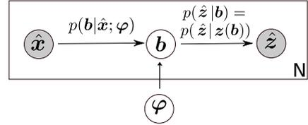
**Fig. 9** Probabilistic graph for the data and physical model based model learning: the shaded nodes are the observed and unshaded are the unobserved (latent) nodes
