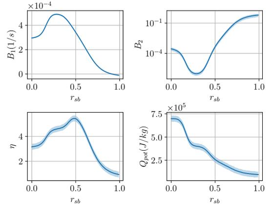
**Fig. 13** Learned probabilistic relation between the hydration model parameters and the slag-binder mass ratio  $r_{sb}$ . Solid line denotes the mean and the shaded  $\pm 2 \times$  standard deviation
