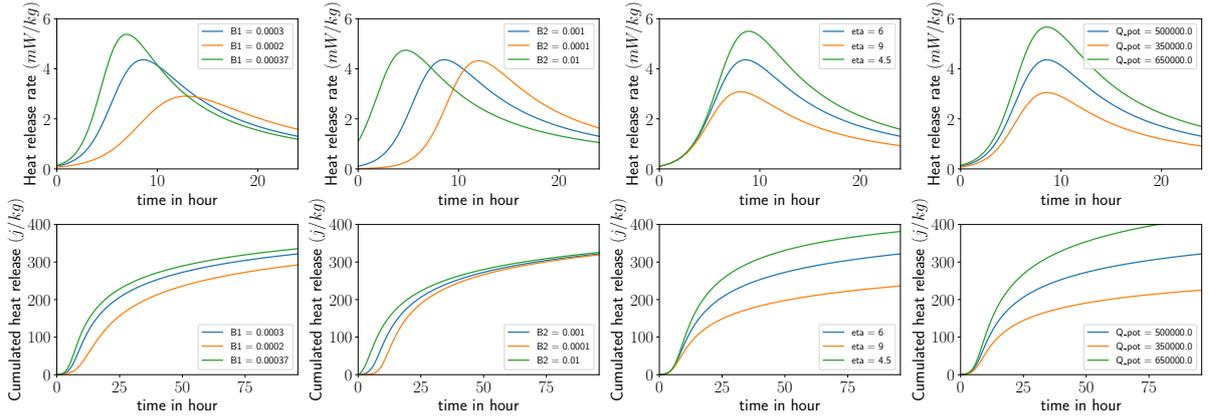
**Fig. B1** Influence of the hydration parameters on the heat release rate and the cumulative heat release.
