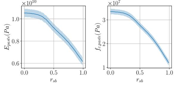
**Fig. 11** Learned probabilistic relation between the homogenization model parameters and the slag-binder ratio  $r_{sb}$ . The solid line denotes the mean and the shaded  $\pm 2 \times$  standard deviation
