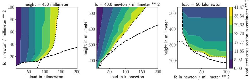
**Fig. 7** Influence of beam height, concrete compressive strength and load in the center of the beam on the required steel. The dashed lines represent the minimum compressive strength constraint Eq. (C46), the dotted lines the geometrical constraint from the spacing of the bars Eq. (C51)
