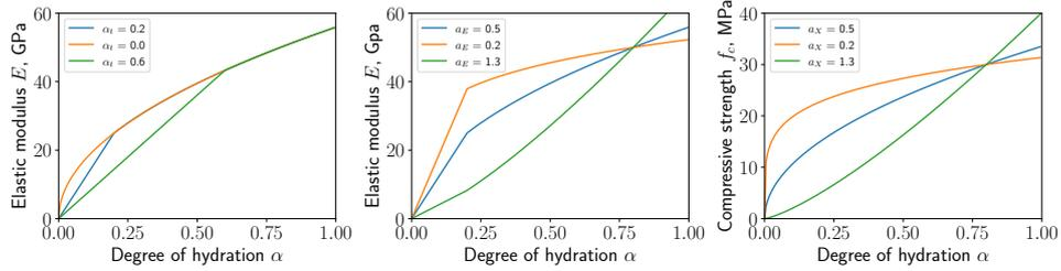
**Fig. 6** Influence of parameters  $\alpha_t$ ,  $a_E$  and  $a_{f_c}$  on the evolution of the Young's modulus and the compressive strength with respect to the degree of hydration  $\alpha$ . Parameters:  $E_{28} = 50$  GPa,  $a_E = 0.5$ ,  $\alpha_t = 0.2$ ,  $a_{f_c} = 0.5$ ,  $f_{c28} = 30$  N/mm<sup>2</sup>,  $\alpha_{28} = 0.8$ .
