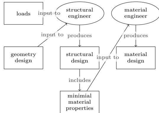
**Fig. 2** Classical design approach, where the required minimal material properties are defined by the structural engineer which is then passed to the material engineer
