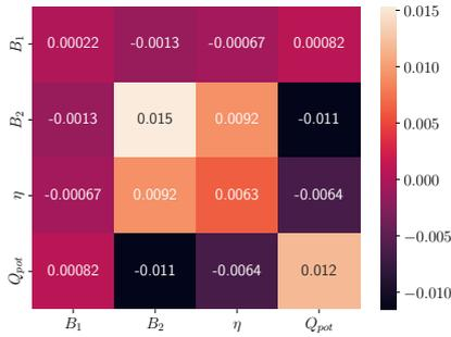
**Fig. 15** Heat map of the converged value of the covariance matrix  $\mathbf{L}\mathbf{L}^T$  of the probabilistic model corresponding to concrete hydration
