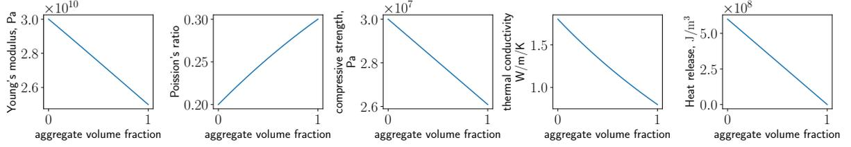
**Fig. 5** Influence of aggregate ratio on effective concrete properties
