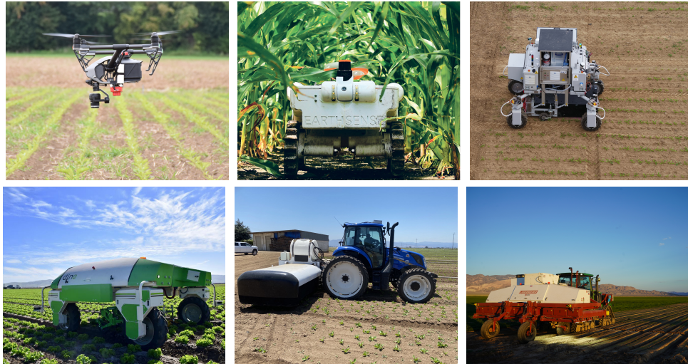
Fig. 2 Unmanned aerial vehicles (UAVs), robots, and smart agricultural machines integrate monitoring, phenotyping, spot-spraying, and chemical-free weeding. Image courtesy: PhenoInspect GmbH, EarthSense, Flourish Project, Naio, Verdant, Carbon Robotics.
