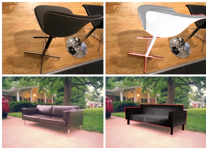
Fig. 1. Given a single input photograph (left) and a known 3D model, our approach accurately estimates the 6D camera-object pose together with the focal length of the camera (right), here shown by overlaying the aligned 3D model over the input image. Our approach handles a large range of focal lengths and the resulting perspective effects.
