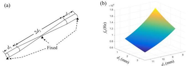
Fig. 3. Schematic diagram of the microcantilever for mechanical mode calculations in the tapered fiber. (b) The resonance frequency of the mechanical modes in the tapered optical fiber varies with the lengths of the untapered ( $d_1$ ) and the tapered regions ( $2d_2$ ).
