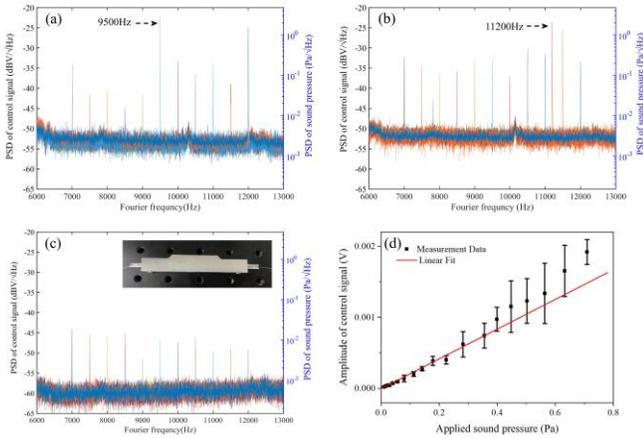
Fig. 2. PSDs of the control signal (PID2) influenced by acoustic waves with different frequency. Different tapered fibers are used in (a) and (b). (c) is the PSD measured after packaging the coupling system and the tapered fiber is the same as used in (a). The inset is the picture of the packaged coupling system. (d) Amplitude of the control signal varies with the sound pressure corresponding to 9500Hz acoustic wave in (a).
