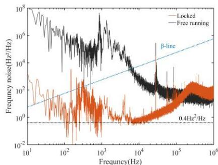
Fig. 4. Laser frequency noise before and after locking.
