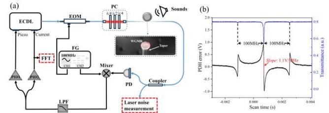
Fig. 1. (a) Experimental setup for laser frequency stabilization and acoustic response monitoring. (b) The PDH error signal and its corresponding WGM transmittance.
