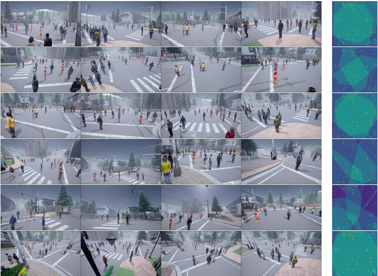
Figure 11. Comparison between camera configurations on Town04crossroad. From top to bottom, we have camera views from Expert 1, Expert 2, Expert 3, random search, max coverage, and the proposed method. We also show FoV coverages and detection results (heatmap overlay) for pedestrians (orange dots).
