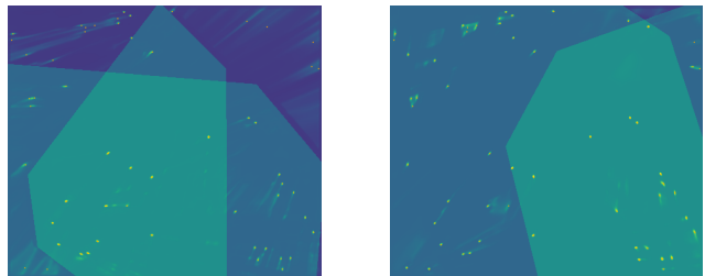
(b) FoV coverage from a human expert (left) vs. our search method (right). Less blue colors indicate the area being covered by more cameras. Zoom in to see the ground truth pedestrian locations (orange dots) and detection results (heatmap overlay).
