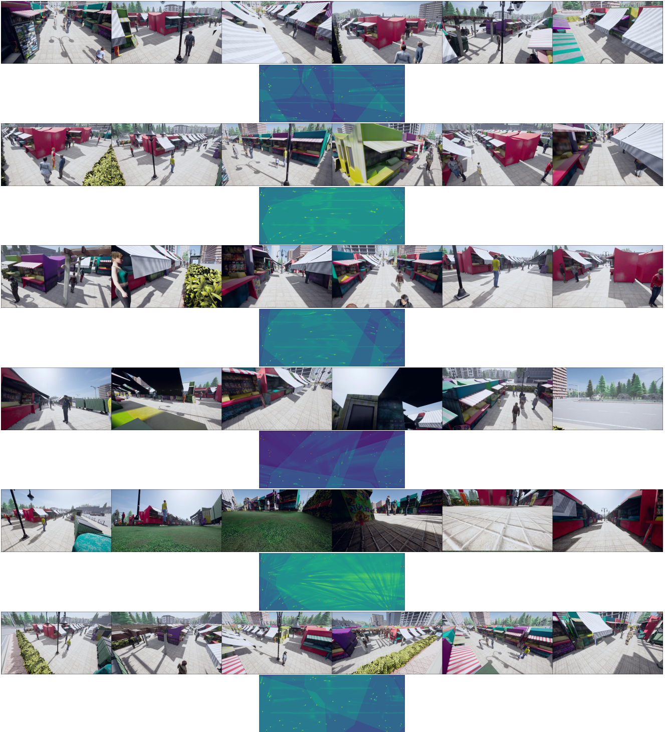
Figure 13. Comparison between camera configurations on Town05market. From top to bottom, we have camera views from Expert 1, Expert 2, Expert 3, random search, max coverage, and the proposed method. We also show FoV coverages and detection results (heatmap overlay) for pedestrians (orange dots).
