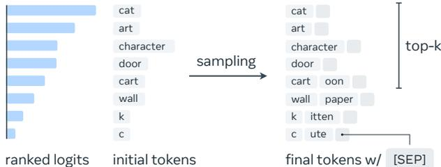
Figure 3. **One-shot sampling** for generating tokens of top- $k$  labels in parallel. Once the model samples the [SEP] token, the label is completed. Otherwise, the model continues for unfinished labels.
