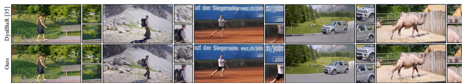
Fig. 7: Visual comparison on DAVIS [56]. We showcase the novel view synthesis results and the corresponding input frame at the same time. DynIBaR [35] may fail to handle some casual videos with few parallax and introduce noticeable artifacts.
