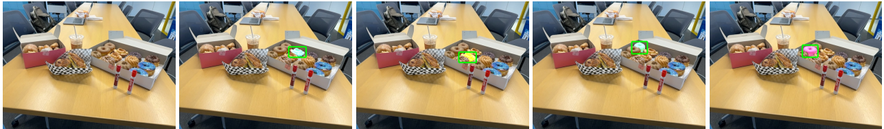
Figure F.2. Examples of Objects with Similar Color. Our method can still distinguish these objects and produce reasonable results in the presence of neighbouring objects with similar appearance, where the Ray-Pair RGB loss is less helpful but remains robust.
