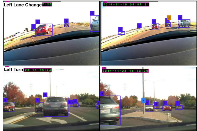
Fig. 3. Object detection pre-processing results on the Brains4Cars dataset [9]. The object classes Car, Bicycle, Person, Traffic Sign, Traffic Light, and Date are mapped to classes 0, 1, 2, 3, 4, and 5 in the images shown.
