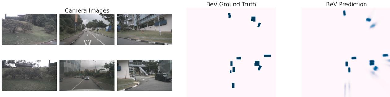
Figure 12. **Qualitative results of PointBeV's prediction on a random sample from the nuScenes validation (not cherry-picked).** The model inputs are the six cameras displayed on the left, respectively the front-left camera, front camera, front-right camera, back-left camera, back camera, and back-right camera. The ground truth and then the prediction are displayed.
