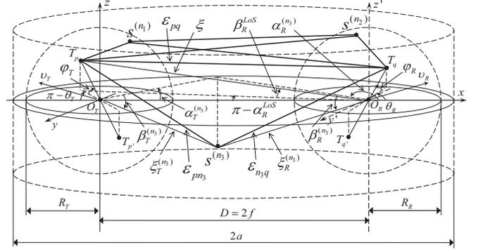
Fig. 1. The proposed 3D MIMO V2V RS-GBSM combining a two-sphere model and an elliptic-cylinder model (only showing the detailed geometry of LoS components and single-bounced rays in the elliptic-cylinder model).
