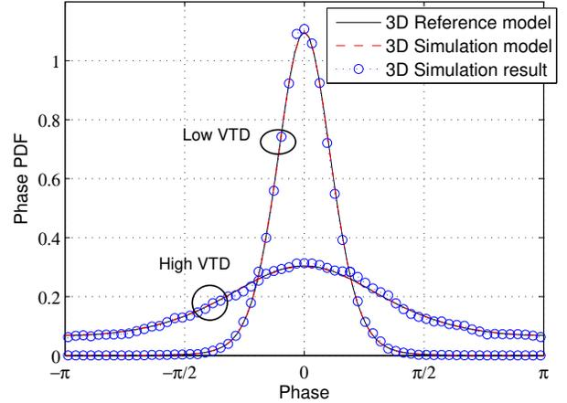
Fig. 5. The phase PDFs for the 3D reference model, 3D simulation model, and 3D simulation result ( $\delta_T = \delta_R = 0$ ,  $\beta_{T0}^{(1)} = 6.7^\circ$ ,  $\beta_{R0}^{(2)} = 17.2^\circ$ ,  $\beta_{R0}^{(3)} = 31.6^\circ$ ).
