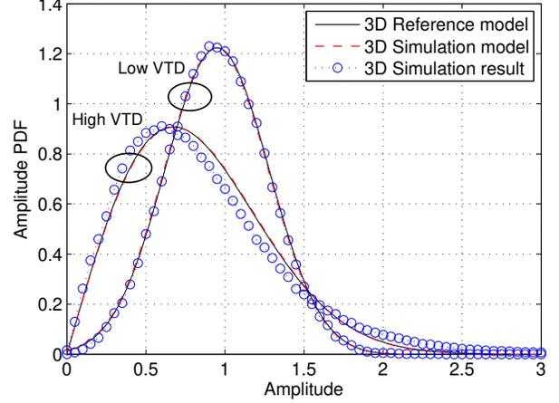
Fig. 4. The amplitude PDFs for the 3D reference model, 3D simulation model, and 3D simulation result ( $\delta_T = \delta_R = 0$ ,  $\beta_{T0}^{(1)} = 6.7^\circ$ ,  $\beta_{R0}^{(2)} = 17.2^\circ$ ,  $\beta_{R0}^{(3)} = 31.6^\circ$ ).
