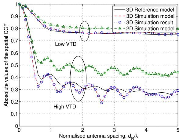
Fig. 7. The absolute values of the spatial CCFs for the 3D reference model, 3D simulation model, 3D simulation result, and 2D simulation model ( $\tau = 0$ , 3D model:  $\beta_{T0}^{(1)} = 6.7^\circ$ ,  $\beta_{R0}^{(2)} = 17.2^\circ$ ,  $\beta_{R0}^{(3)} = 31.6^\circ$ , 2D model:  $\beta_T^{(n1)} = \beta_R^{(n2)} = \beta_R^{(n3)} = \beta_{T0}^{(1)} = \beta_{R0}^{(2)} = \beta_{R0}^{(3)} = 0^\circ$ ).
