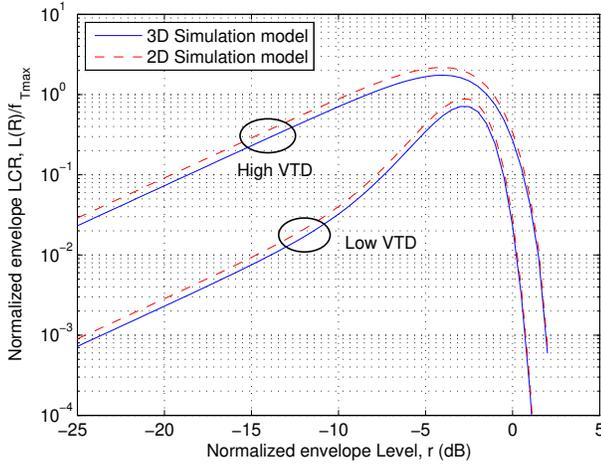
Fig. 9. The normalized envelope LCRs for the 3D and 2D simulation models (3D model:  $\beta_{T0}^{(1)} = \beta_{R0}^{(2)} = \beta_{R0}^{(3)} = 60^\circ$ , 2D model:  $\beta_T^{(n1)} = \beta_R^{(n2)} = \beta_R^{(n3)} = \beta_{T0}^{(1)} = \beta_{R0}^{(2)} = \beta_{R0}^{(3)} = 0^\circ$ ).
