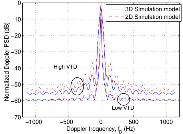
Fig. 8. The normalized Doppler PSDs for the 3D and 2D simulation models ( $\delta_T = \delta_R = 0$ , 3D model:  $\beta_{T0}^{(1)} = 6.7^\circ$ ,  $\beta_{R0}^{(2)} = 17.2^\circ$ ,  $\beta_{R0}^{(3)} = 31.6^\circ$ , 2D model:  $\beta_T^{(n1)} = \beta_R^{(n2)} = \beta_R^{(n3)} = \beta_{T0}^{(1)} = \beta_{R0}^{(2)} = \beta_{R0}^{(3)} = 0^\circ$ ).
