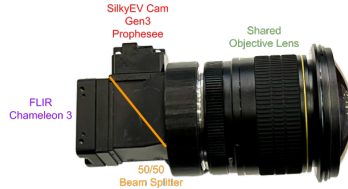
Figure 10. Constructed single objective beam splitter with each major component labeled. As constructed the Event Camera will be flipped compared to a traditional setup.
