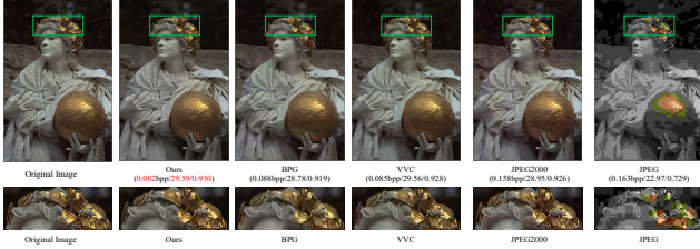
Figure 6. Visualization of reconstructed images and enlarged images of kodim17 from Kodak dataset.
