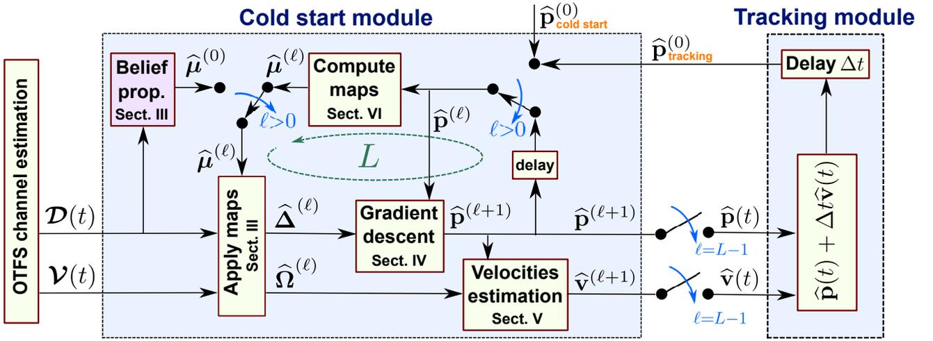
Fig. 2. Scheme of the TIP algorithmic framework. The switch on the left-hand side of the Cold start module remains in place for all  $\ell \geq 0$  in the Tracking mode, since the Belief propagation block is unused.
