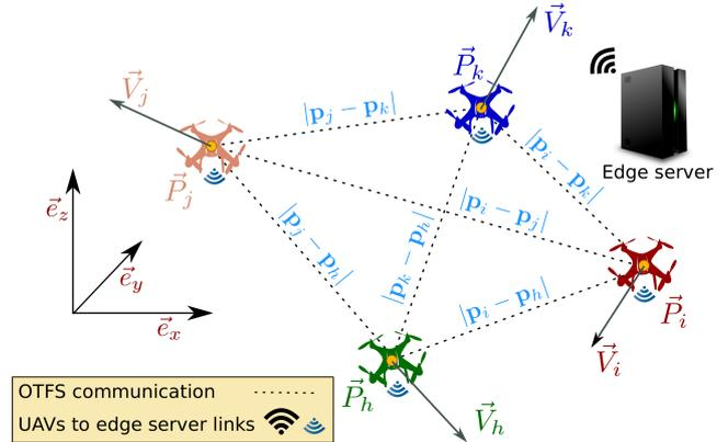
Fig. 1. Communicating UAVs assisted by an edge server. The  $n$ -th UAV has position  $\vec{P}_n$  and velocity  $\vec{V}_n$ , measured with respect to a common Cartesian coordinate system. The notation  $|\mathbf{p}_n - \mathbf{p}_m|$  denotes the distance between UAV  $n$  and UAV  $m$ , where  $\mathbf{p}_n$  and  $\mathbf{p}_m$  are the components of the geometric vectors  $\vec{P}_n$  and  $\vec{P}_m$ , respectively.
