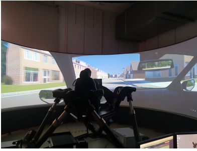
Fig. 2. An example of 6-DOF driving simulator for LFT installed at Technical University of Munich
