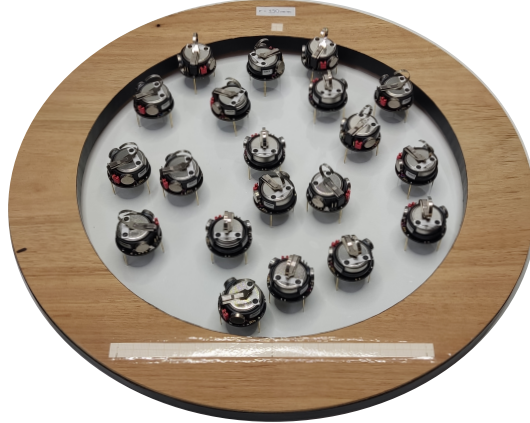
FIG. 1. Experimental setup. 20 Kilobots were positioned within a circular arena with a radius of 15 cm. The labels used to track the orientation of the particles are visible in the picture.
