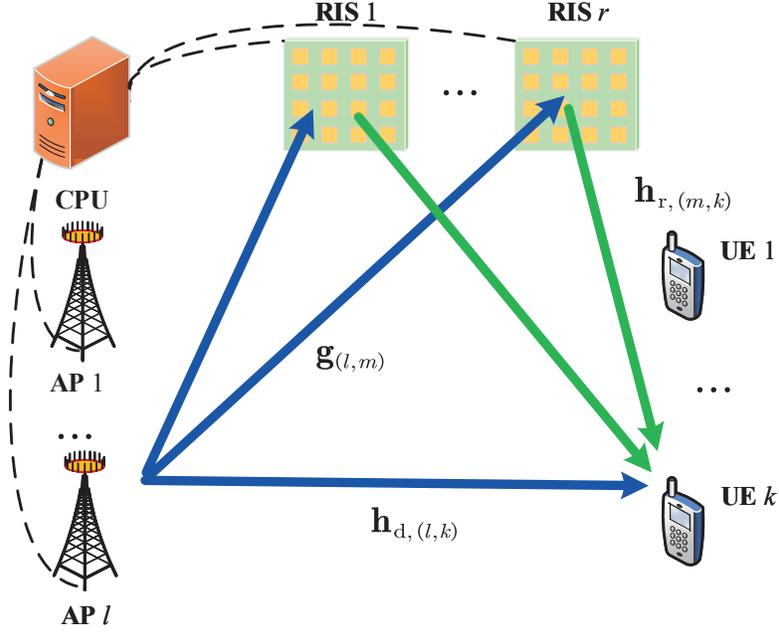
Fig. 1. System block diagram of a general RIS-aided cell-free network.
