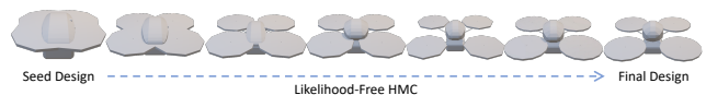
Figure 6: Sub-sampled quadcopter designs taken along the likelihood-free HMC chain using DNRE. The initial seed design on the far left has multiple structural interferences, including sensors that cut through the fuselage. As we move along the chain we see the design morph into our desired structure with very few interferences. This is achieved through increasing the arm length and changing the shape of the fuselage, as well as varying the placement of the interior sensing components.
