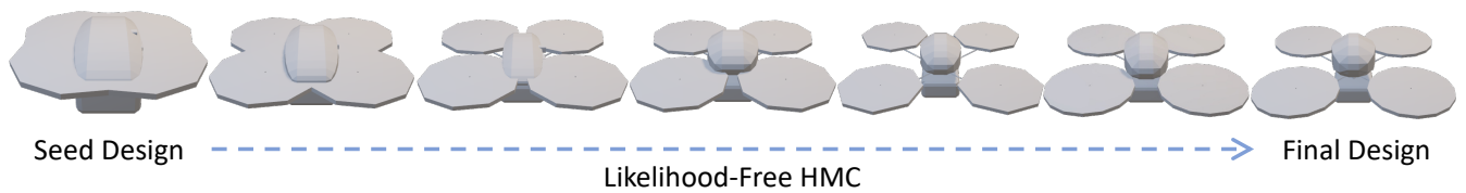
Figure 11: Sub-sampled quadcopter designs taken along the likelihood-free HMC chain using DNRE. The initial seed design on the far left has multiple structural interferences, including sensors that cut through the fuselage. As we move along the chain we see the design morph into our desired structure with very few interferences. This is achieved through increasing the arm length and changing the shape of the fuselage jointly with varying the placement of the interior sensing components.
