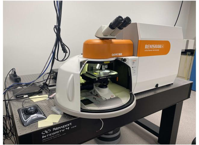
FIG. 1. Digital photograph of the Renishaw inVia™ confocal Raman microscope used in our experiments.
