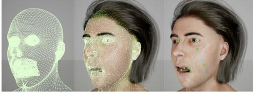
Figure 2. Template model used to create SPHEAR. From left to right, the base geometry including the tongue, eyeballs, and teeth, the hair, the template mesh connectivity, and the kinematic rig (joints).
