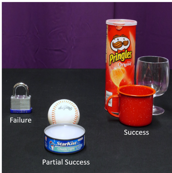
Fig. 10: This figure shows the YCB objects we evaluated the TRL gripper against. All of the items were chosen to be above the maximum demonstrated capacity for the Pneu-net gripper so any objects grasped show added capability. Additionally we filtered to non-box objects that fit within the jaws of the TRL gripper. Of these items, the TRL lifted five items successfully, with two being partial successes. The only failure is the padlock.
