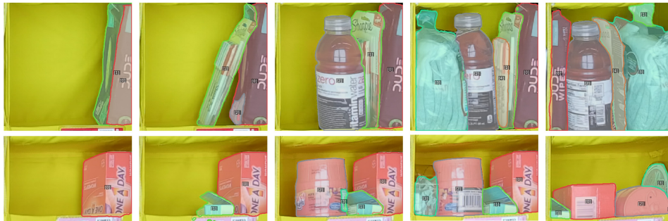
Figure 4: Visualized results for the shelf environment. Masks with the same color and index are associated and predicted as the same object by the network.
