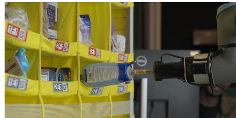
Figure 1: A densely packed shelf environment. The shelf holds objects from a wide array of categories. During the stowing process, a human operator may obscure the camera’s view and rearrange the objects within the bin. The robot’s task is to pick a specific object as directed by the given order index of the object’s placement in the bin.
