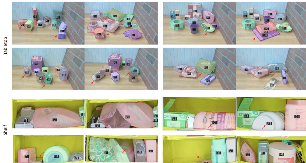
Figure 10: Failure Cases Illustrated. In the Tabletop settings (top 2 rows), we observe under-segmentation (top left), over-segmentation (top right), mismatch (bottom left), and mistrack (bottom right). In the Shelf settings (bottom two rows), the failures include a combination of under-segmentation and failure to detect new objects (top left), failure to track and mismatch (top right), failure to detect (bottom left), and failure to segment (bottom right).
