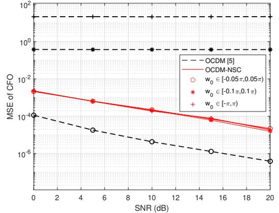
Fig. 1: MSEs of CFO estimators versus SNR
