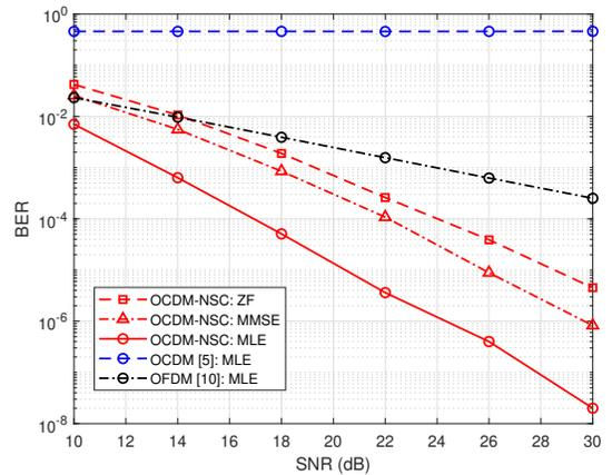
Fig. 2: BER performance with the proposed CFO estimator
