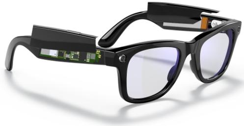
Figure 1. **Smart Glasses with Electronics**: The designed smart glasses hardware. The left hanger holds the miniaturized electronics. The right hanger contains the battery, with an energy content of up to 154mAh.
