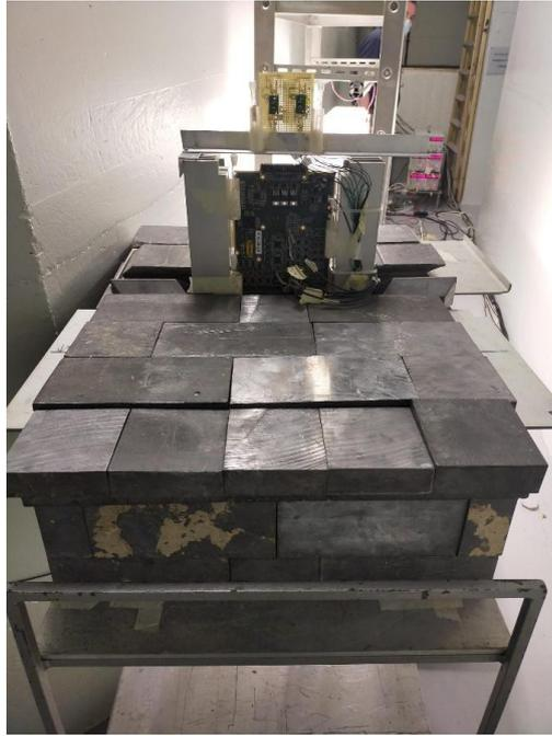
Figure 43 - Photo of the lead screen used for irradiation tests.
