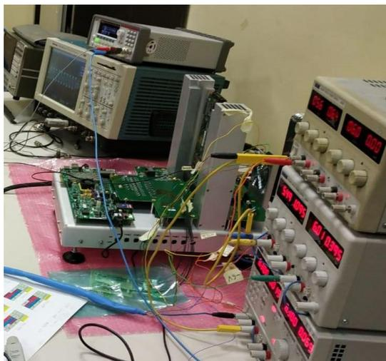
Figure 46 - Set up used for calibration measurements. This picture shows the APU board mounted on the APU\_ADAPTER and the Xilinx evaluation board which allowed the controls and DSP.
