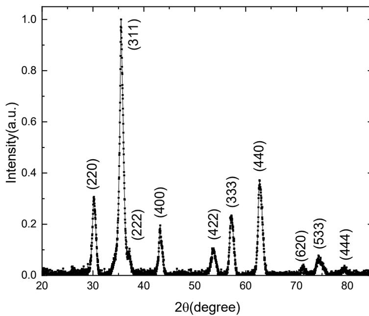
Figure S1. X-ray diffraction pattern of the Fe<sub>3</sub>O<sub>4</sub> as-synthesized nanoparticles where the diffraction peaks are indexed with the Fd3m space group of the Fe<sub>3</sub>O<sub>4</sub> spinel.
