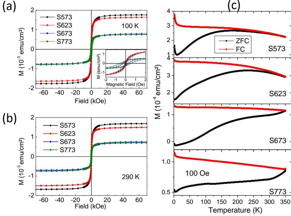
Figure 5. Magnetization as function of the field at 100 K(a) and 290 K(b) and ZFC-FC curves (c) of the samples annealed at different temperatures. Inset in (a) is a zoom of the magnetization at low field.
