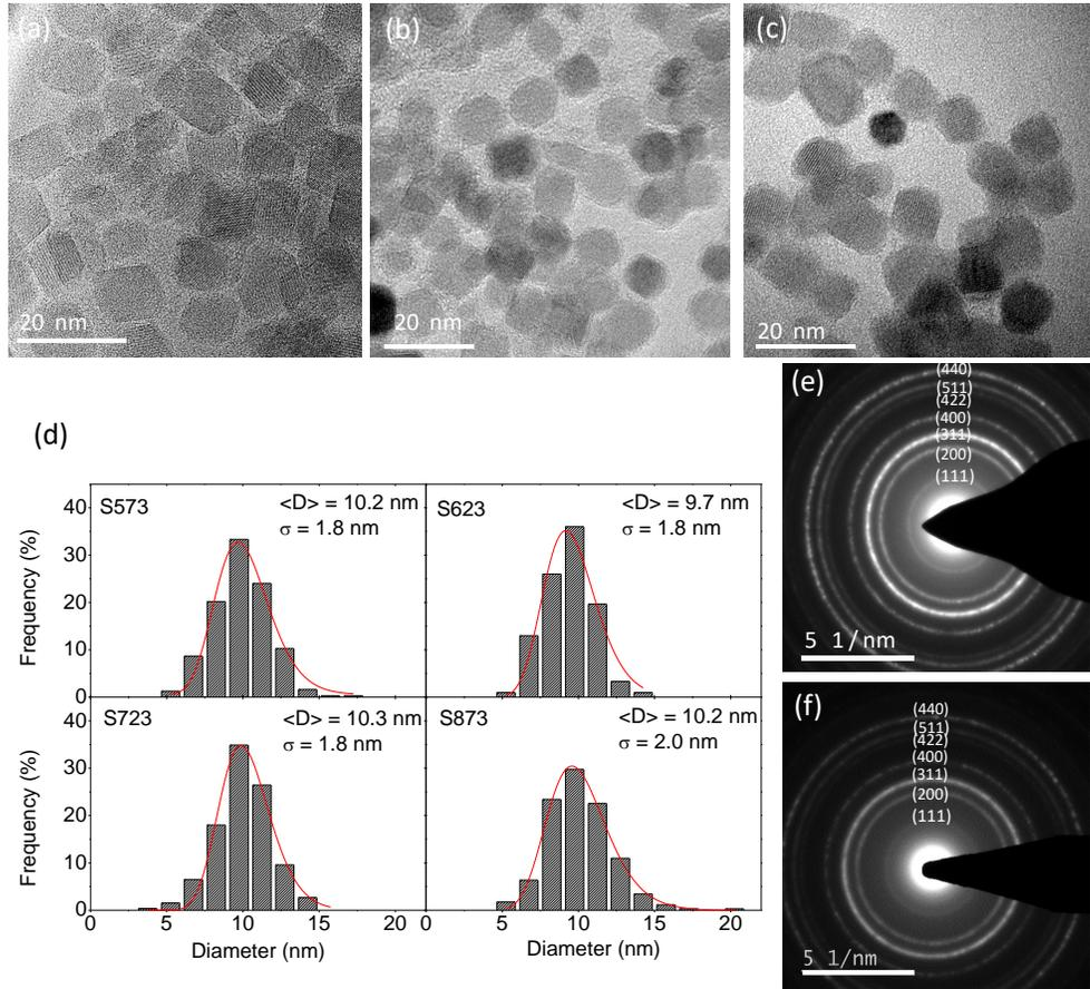
Figure 2. TEM images of the samples S573 (a), S723 (b) and S873 (c) and the corresponding size distribution are shown in (d), where the red line is the fit with a lognormal distribution. Electron diffraction of the sample S573 (e) and S873 (f), where the spinel diffraction rings are indicated.
