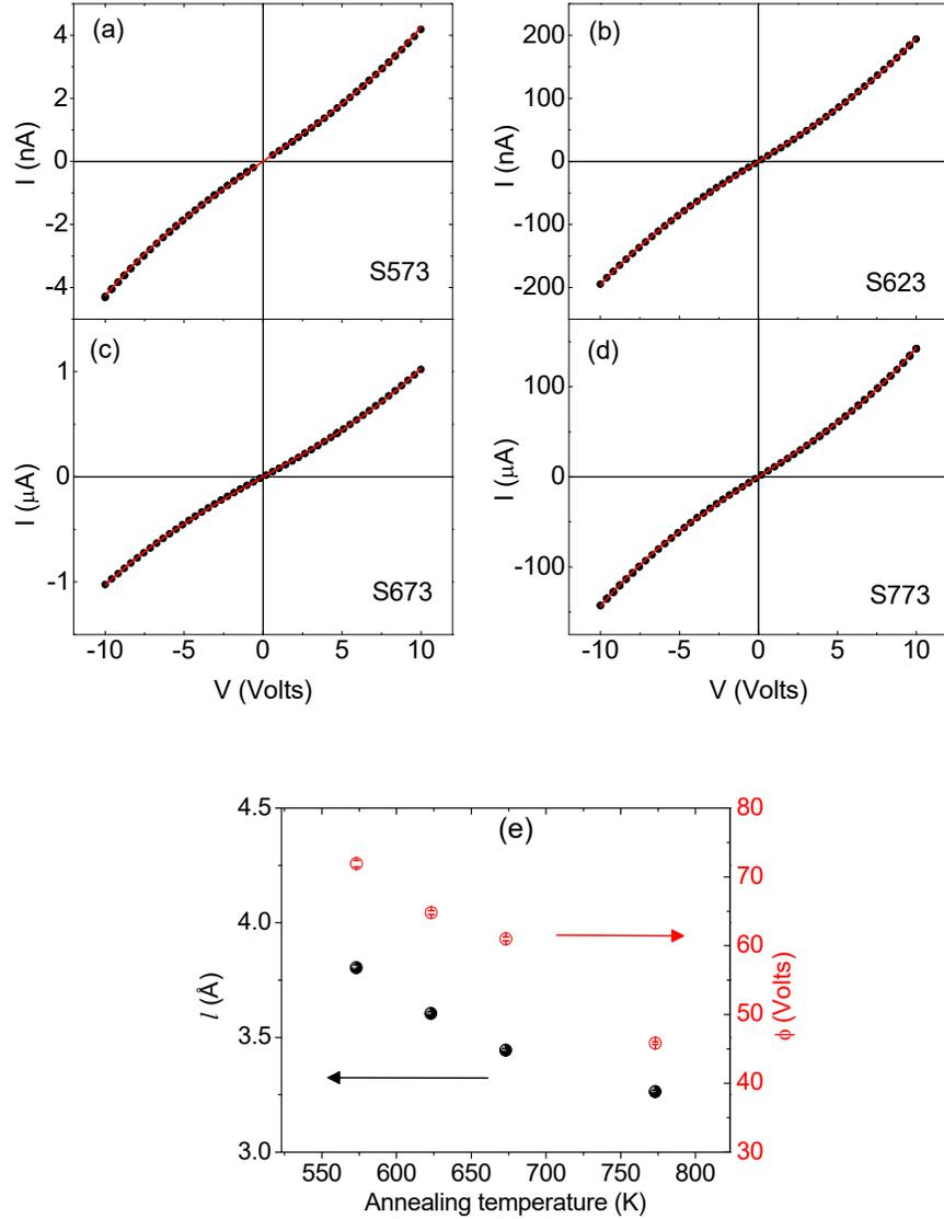
Figure 6. Current-voltage curves measured at 100 K for the samples S573 (a), S623(b), S673(c) and S773(d). The red line is the fit of experimental data to equation (1). The values of  $l$  and  $\phi$  obtained from the fits are plotted as a function of the annealing temperature in (e).
