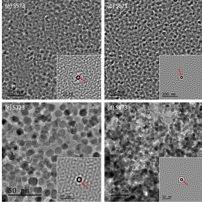
Figure 3. Low magnification TEM images of the self-assemblies annealed at 573 K (a), 625 K (b), 723 K (c) and 873 K (d). The inset shows the auto-correlation image of each figure. The red line indicates the position of intensity analysis.
