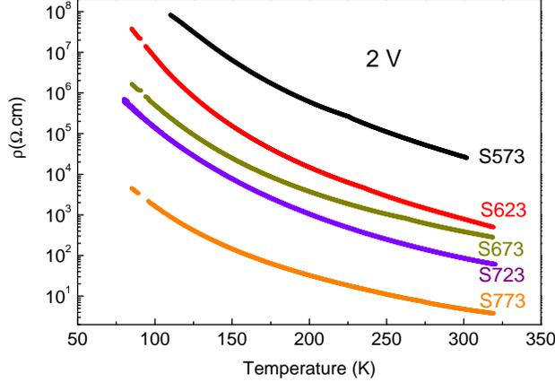
Figure 7. Resistivity as function of temperature measured with an applied voltage of 2 V for all annealed self-assemblies.
