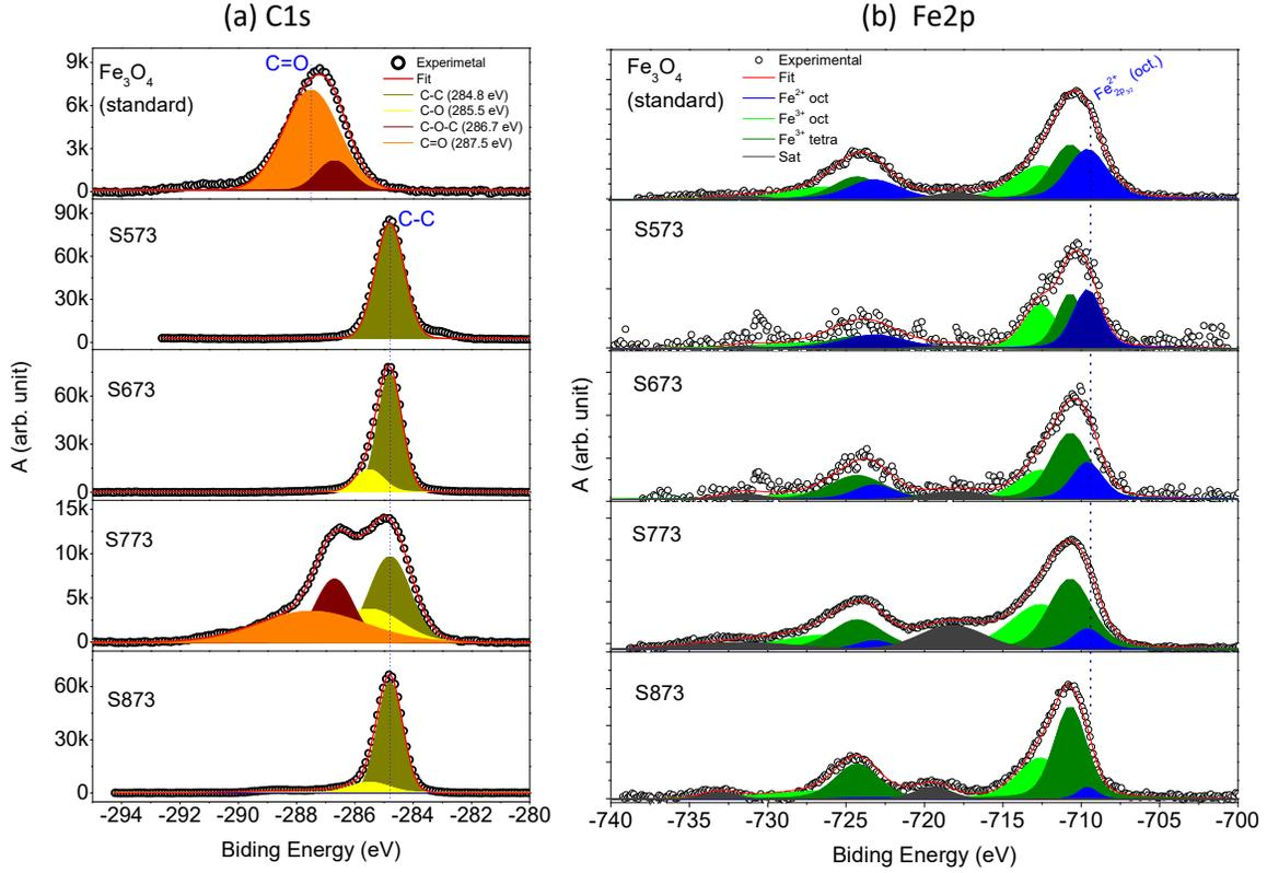
Figure 4. Background subtracted XPS spectrum in the C1s region (a) and Fe2p region (b) of  $\text{Fe}_3\text{O}_4$  pattern sample and nanoparticles self-assemblies with the corresponding fitting curves (red line). The blue dotted vertical line marks the position of the  $\text{Fe}_{2p_{3/2}}^{2+}$  peak.
