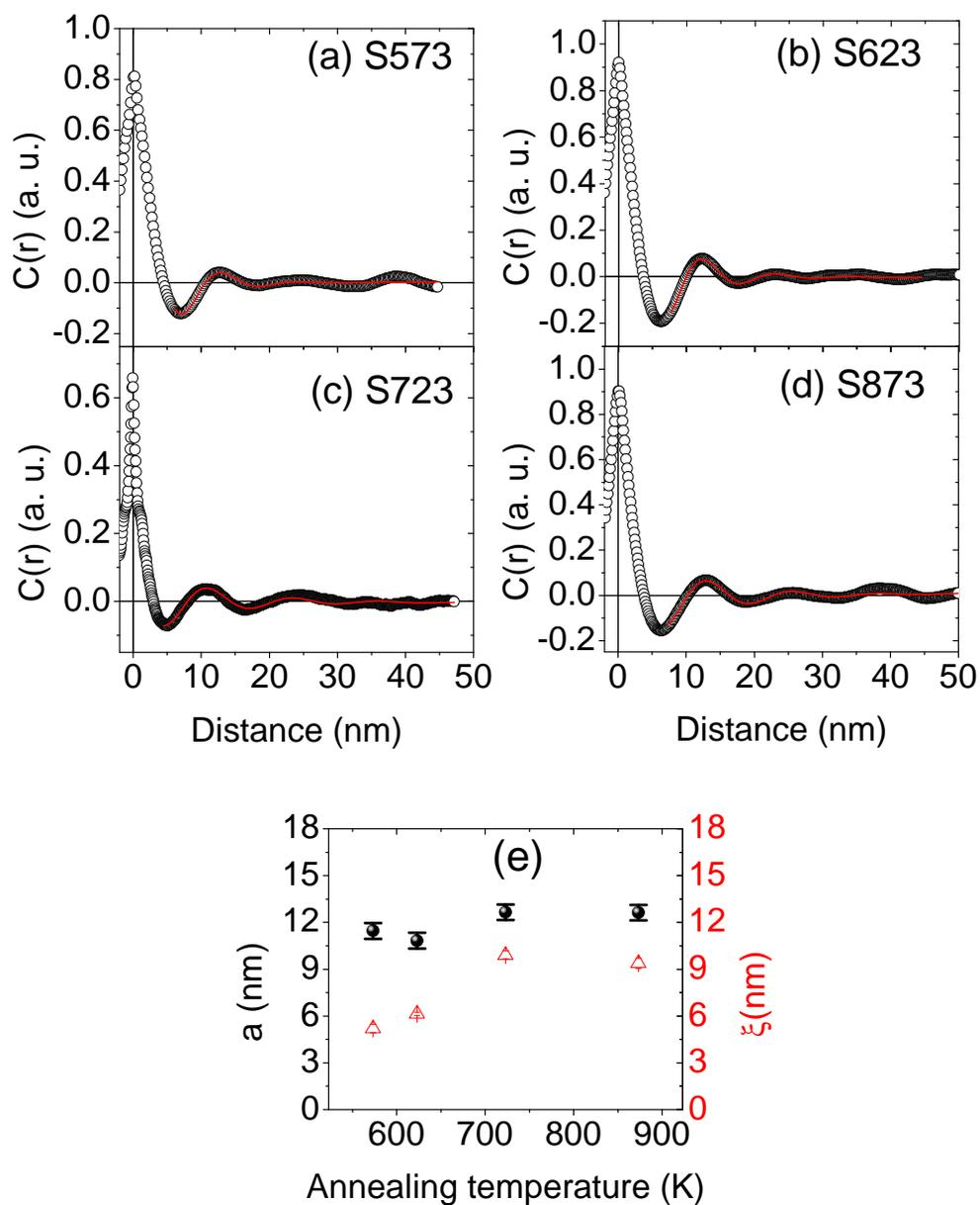
Figure S2. Radial profile of the autocorrelation spectrum extracted along the red lines presented in the figure 3 for the self-assemblies annealed at 573 K (a), 623 K (b), 723 K (c) and 873 K (d). The red line is the fit equation using the equation given in the text. In (e) is shows to adjusted  $\xi$  and  $a$  parameters as function of the annealing temperature.
