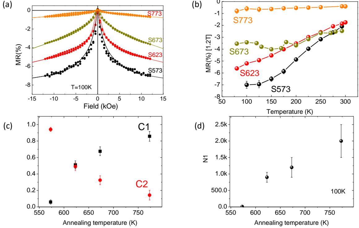
Figure 8.  $MR$  at 100 K (a) and the temperature dependence of the  $MR$  at 12 kOe (b) for the samples annealed at different temperatures. The solid lines in (a) are the fit of  $MR$  with the magnetic loops and scattering through non-collinear surfaces spin described by a Langevin function. The adjusted C1 and C2 parameters are presented in (c) and N1 in (d) as function of the annealing temperature.
