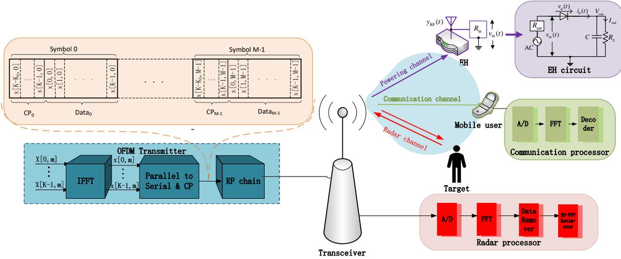
Fig. 1. System and OFDM Signal Model for ISCAP.
