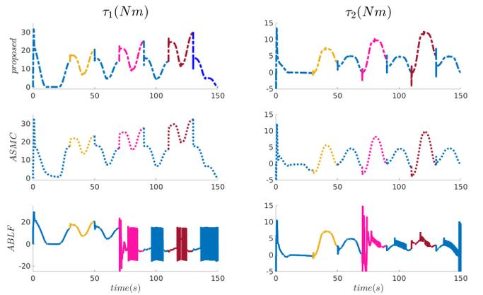
Fig. 6. Torque inputs  $\tau_1, \tau_2$  generated by the controllers for the respective joints. The blue lines represent the unloaded period; the yellow lines represent the period with the first payload; the pink lines represent the period with the second payload, and the brown lines represent the period with the third payload.
