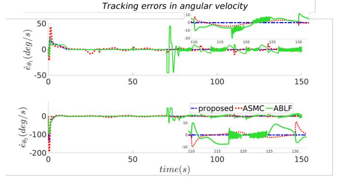
Fig. 5. Errors in angular velocities  $\dot{\theta}_1, \dot{\theta}_2$ . The proposed controller ensures that the errors stay within the bounds.
