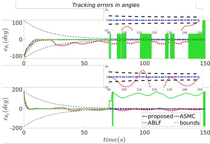
Fig. 4. Errors in angles  $\theta_1, \theta_2$ . The proposed controller ensures that the errors stay within bounds.
