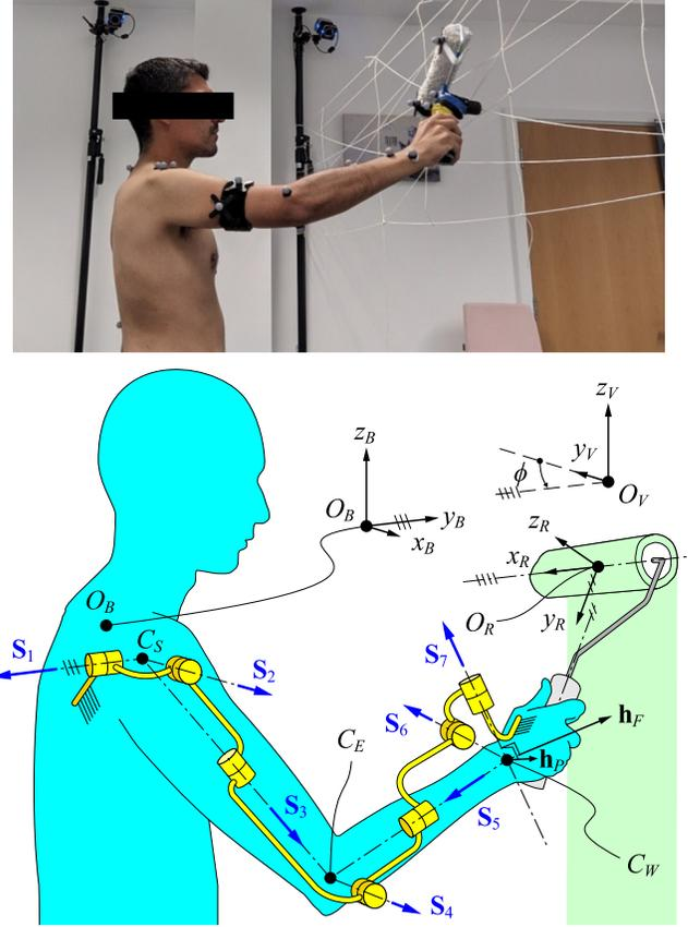
Fig. 14. Data collection for experiment VI-D. TOP: A participant demonstrates how he holds a roller against a wall. The wall is a net of threads to allow the cameras track the markers. The markers set is defined for tracking of the joint centres, and thorax and roller frames. BOTTOM: Kinematic model and related coordinate systems for right arm holding a paint roller.
