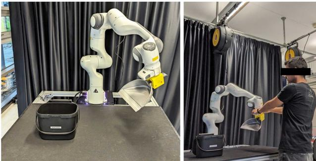
Fig. 6. LEFT: Setup for experiment in Sec. VI-C – a Franka Panda arm with a dustpan as end-effector, and a bin on the table. RIGHT: A participant carries out a kinesthetic demonstration.
