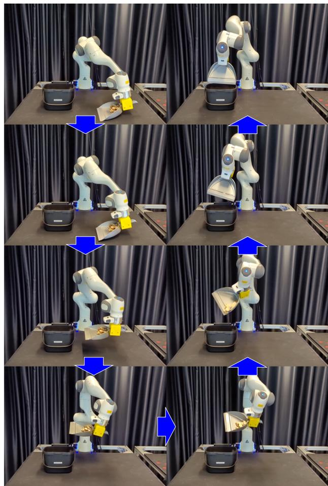
Fig. 9. Franka Panda arm following the mean task-space trajectory obtained from  $\mathcal{D}$ . See video in the supplementary material.
