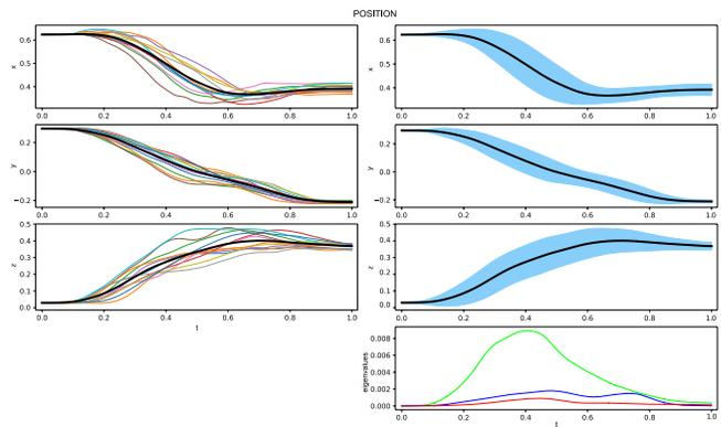
Fig. 8. LEFT: Positions of demonstrations  $\mathcal{D}$ , i.e. dataset  $\{\{(\mathbf{p}_{ij}, t_{ij})\}_{j=1}^{M_i}\}_{i=1}^N$ ,  $\mathbf{p}_{ij} = (x_{ij}, y_{ij}, z_{ij}) \in \mathbb{R}^3$ . RIGHT: Mean  $\hat{\boldsymbol{\mu}}(t)$  with 1.5 standard deviation density level. RIGHT-BOTTOM: eigenvalues of  $\hat{\boldsymbol{\Sigma}}(t)$
