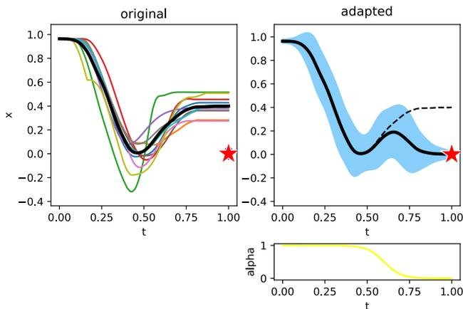
Fig. 17. Adaptation of a scalar model to a desired final point that is outside the training data. The data are  $N = 10$  trajectories. The desired point is  $x^* = 0$  at  $t^* = 1$  with  $\sigma^* = 0.01$ . The chosen parameters are  $g = 0.25$ ,  $S = N$ ,  $\alpha(t) = 0.5 - 0.5 \tanh(10(t - 0.6))$
