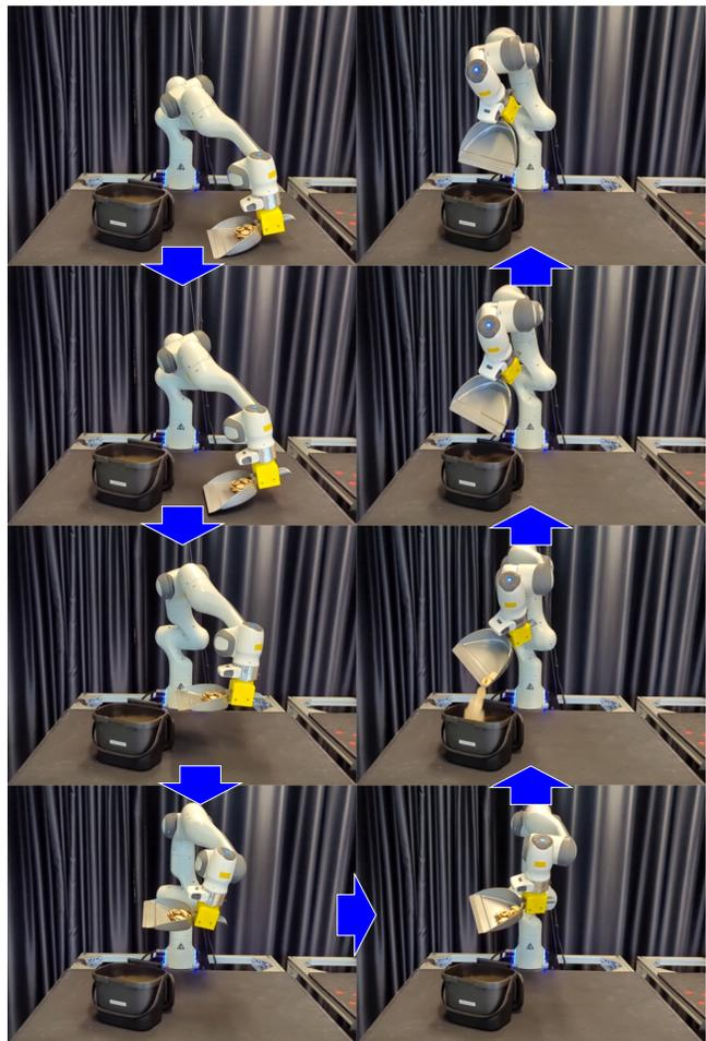
Fig. 12. Franka Panda arm following the adapted task-space trajectory after the bin has been moved. See video in the supplementary material.
