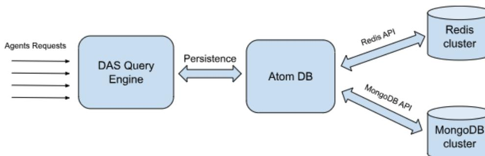
Figure 2: High level architecture of Hyperon Distributed Atomspace
