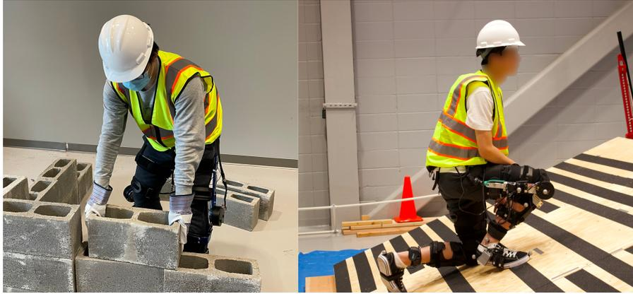
Figure 3: Modern robot embodiment includes exoskeletons. Flexible, light-weight, high-torque bilateral knee exoskeletons are shown here in the task of assisting construction workers to reduce fatigue and injuries. Left: Masonry work. Right: Roof worker with kneeling gait (14).
