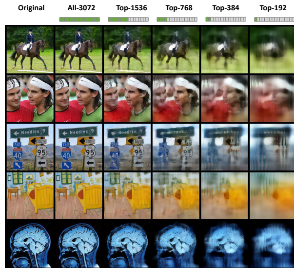
Figure 12: Reconstruction from top principle components: The top- K principle components correspond to the largest K eigenvalues of the covariance matrix computed from 50,000 image embeddings in the ImageNet validation set. With a selection of top-192 components (the right column), the color and layout of the images are primarily determined, but the resulting reconstructions appear blurred with noticeable loss of details. As more principle components are incorporated, the finer details are gradually restored. Best viewed in color.
