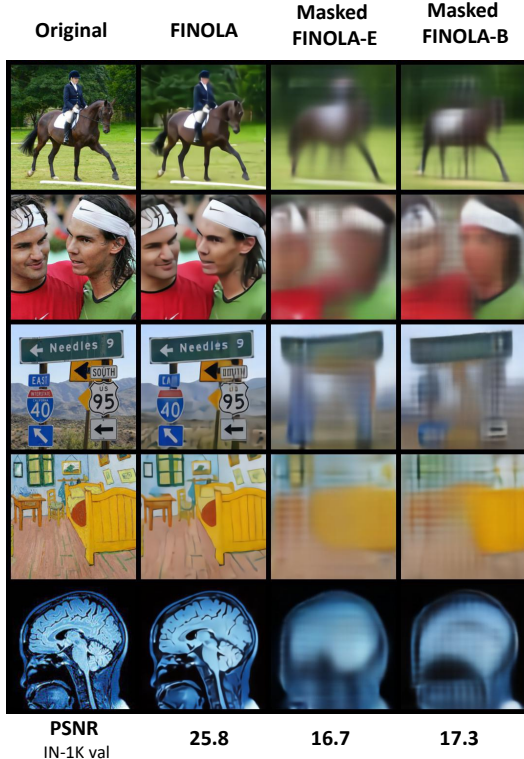
Figure 19: FINOLA vs. masked FINOLA on image reconstruction: In this comparison, the encoders of the two masked FINOLA variants are frozen, and their attentional pooling and FINOLA components are fine-tuned. To ensure a fair comparison, we replace the decoders in the masked FINOLA variants with the same architecture as FINOLA, trained from scratch. When compared to vanilla FINOLA, the masked variants preserve color and shape information but exhibit a loss of texture details.
