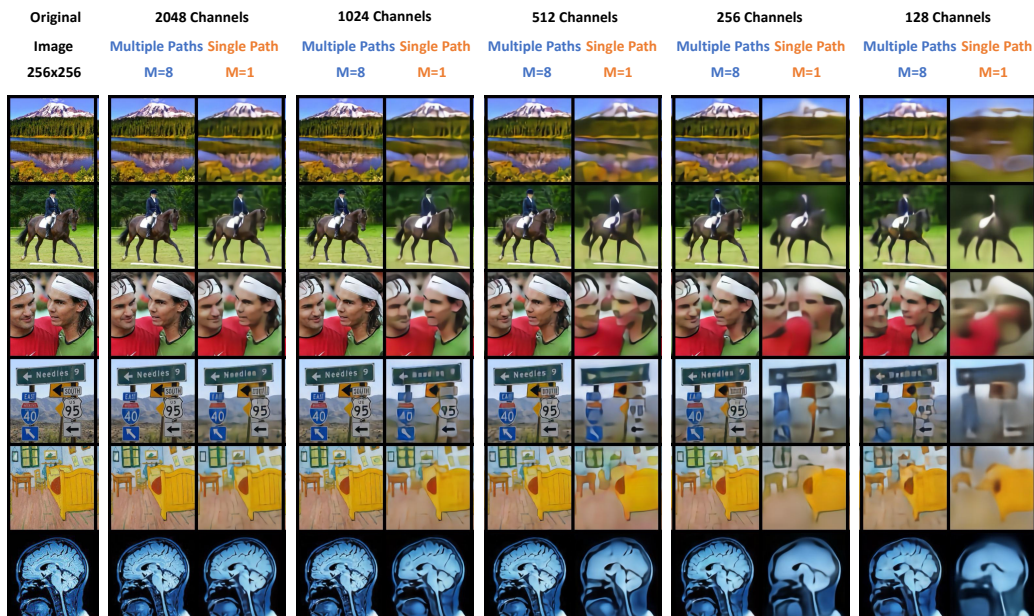
Figure 13: Multiple paths vs. Single path: Summing M = 8 FINOLA solutions \phi_i (as in Eq. 3) yields superior image reconstruction quality compared to the single path counterpart. This trend holds across various dimensions (from C = 128 to C = 2048 ). Resolution of feature map z is set to 64 \times 64 , with an image size of 256 \times 256 . Best viewed in color.
