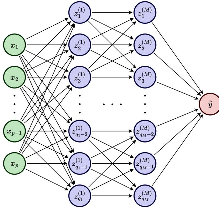
**Figure 1:** Structure of a feed-forward neural network with  $p$ -dimensional input layer, hidden layers  $z^{(1)}, \dots, z^{(M)}$ , with  $q_1, \dots, q_M$  nodes, respectively. The network has a single output node  $\hat{y}$ .
