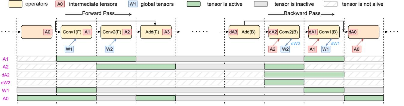
**Figure 6: An example of tensor vitality analysis for a residual basic block. Operators in forward propagation and in backward propagation are marked as Op(F) and Op(B), respectively.  $A_x$  and  $W_x$  are activation tensors and weight tensors, respectively.  $dA_x$  and  $dW_x$  are the corresponding gradient tensors.**
