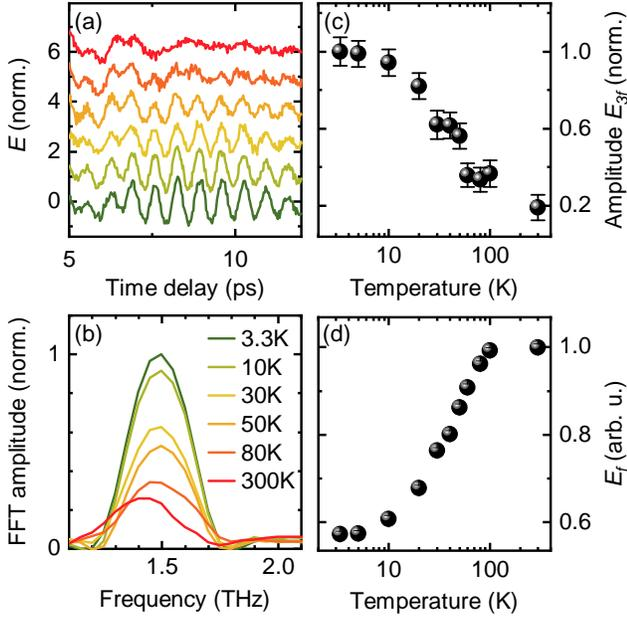
Figure 2. (a) THG signal in time domain at different temperatures. (b) Fourier amplitude of the signal in panel (a). (c) THG amplitude  $E_{3f}$  as a function of temperature. (d) The transmitted amplitude  $E_f$  of the fundamental frequency.
