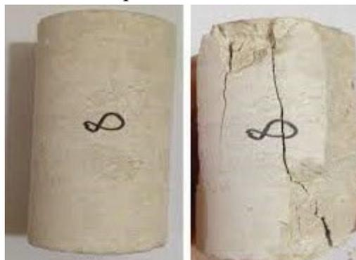
**FIGURE 9. Typical failure modes of cylindrical specimen in conventional triaxial test**
