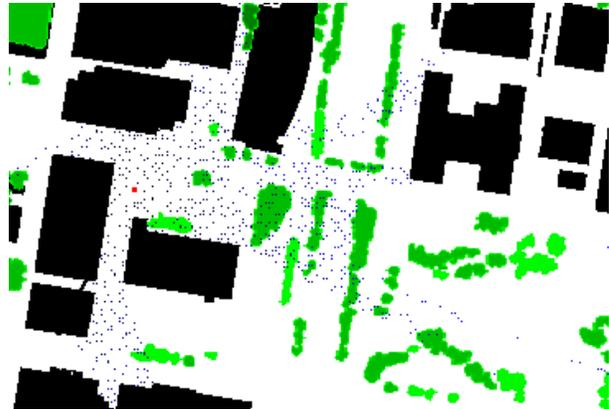
Fig. 2: An example of the dataset for a single pole showing building footprints in black, foliage heights through green shades, the pole location in red, and receiver locations in blue.
