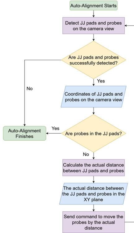
Figure 6: Flowchart Diagram of the Auto-alignment Process
