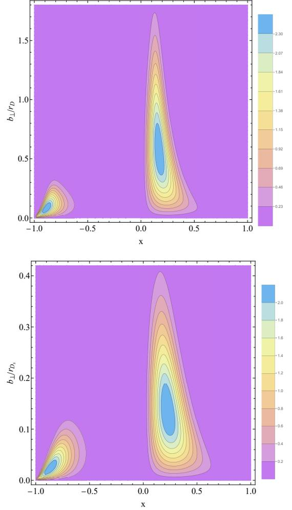
FIG. 8. Impact parameter space GPDs. For illustrative purposes, we have considered the convenient representation of Eq. (50), where the quark lies in the  $x > 0$  domain, while the antiquark in  $x < 0$ . *Upper panel:*  $D$ -meson results. *Lower panel:* analogous results for the  $D_s$  meson. The conspicuous asymmetry in both cases is due to the difference in mass of the dressed valence quarks: the heavy quark plays a larger role in determining the center of transverse momentum.
