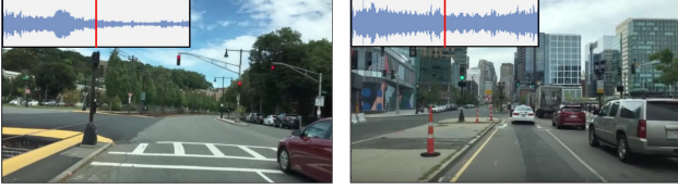
Figure 3: Illustration of the Importance of Audio. The frame is consistent with the red arrow marked on the waveform. Left: audio amplitude decreases and maintains a low level when the vehicle is going to wait for traffic lights. Right: audio experiences many ups and downs representing acceleration and brake in a narrow urban area.
