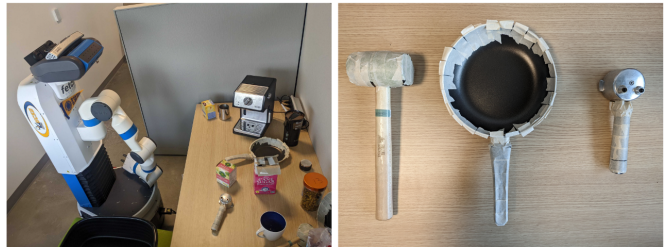
Fig. 6. Left: the setup of the real-world experiment with Fetch. Right: Objects (hammer, pan, and espresso machine handle) used in the real-world experiment.
